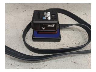
4. Insert the battery into the holder on the receiver. Upon insertion of the battery, the trailer board will run through a start-up sequence so you can check that all lights work before operating.
