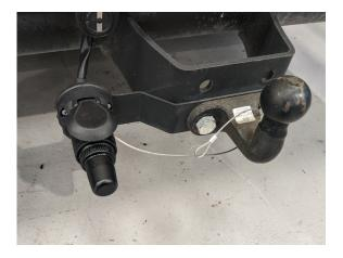
1. Plug the transmitter into the trailer plug.
