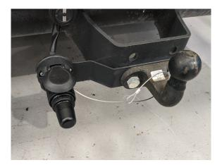
1. Plug the transmitter into the trailer plug on the patrol vehicle.
