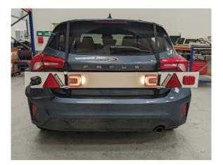
7. Please keep the side lights on for the entire duration of using the Wireless Trailer Board kit to ensure a continuous signal between the transmitter and receiver.
