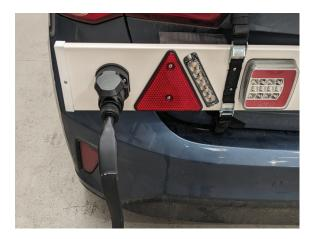
3. Plug the lead (on the receiver/ battery holder) into the trailer board.
