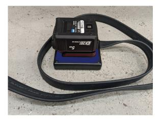
5. Insert the battery into the battery holder on the receiver. Upon insertion of the battery, the trailer board will run through a start-up sequence so you can check that all lights work before operating.
