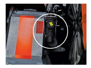
8. Plug the transmitter into the supplied adapter and insert the transmitter (with the adapter attached) into the trailer socket on the RDT.
