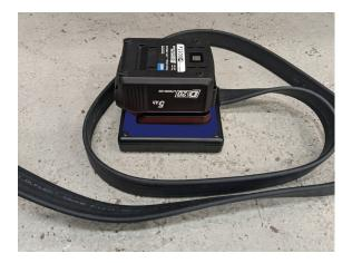
4. Insert the battery into the battery holder on the receiver. Upon insertion of the battery, the trailer board will run through a start-up sequence so you can check that all lights work before operating.
